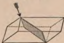
Nicol prism: original form: arrow shows crystallographic axis.
